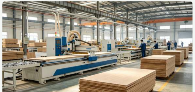
Cabinetry production line – CNC cutting, edge banding and QC before packing
